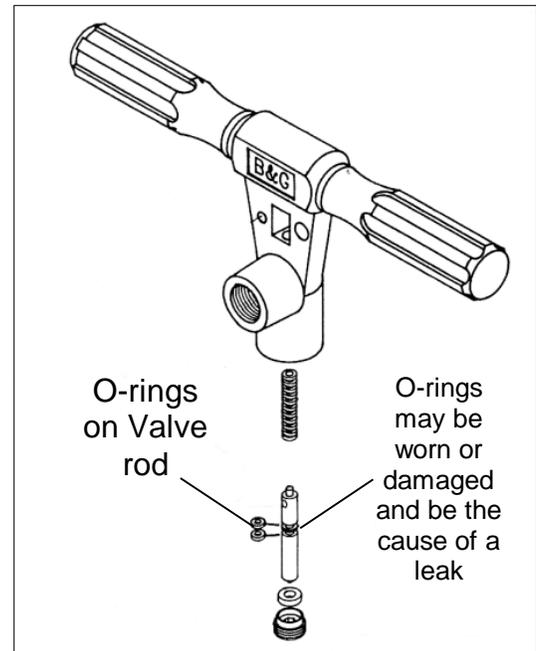
**P.** Leaking occurs around the rod spring at the center of the valve handle.
